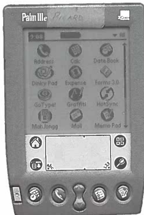
Figure 1a. Palm Computing Inc.'s model IIIe. Touch sensitive LCD screen measures 5.7 x 7.8 cm.
