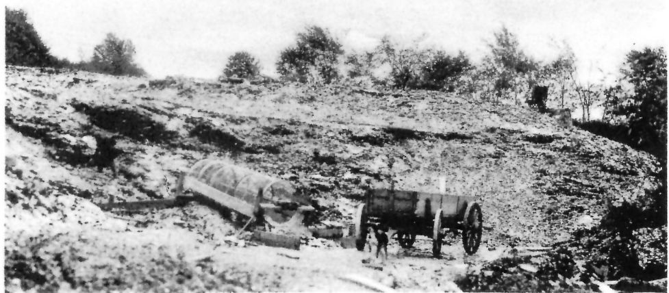
B. Portion of large dump, containing thousands of tons of shop-scrap mica, at Lacey mine, concession VII, lot 11, Loughborough township, Ont. The material of this dump, representing the accumulated waste from the trimming shop, is passed through the gasoline-driven screen, the oversize being shipped for grinding
