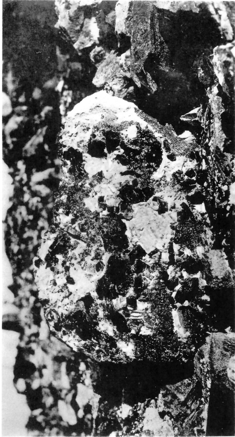
Mass of vein-filling from a mica lead, concession VI, lot 13, North Burgess township, Ont. Illustrates the typical mode of occurrence of phlogopite crystals disseminated throughout a matrix of pink calcite in deposits of the pocket type.
