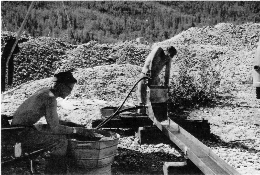
FIGURE 14. Concentrating unit showing aluminum feed box and sluice boxes. Operator at left is panning sluice tailings to check recovery efficiency of unit.
